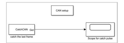
If you send CAN bus data frame with CAN ID =44 (11 bits CAN ID) and 8 Data bytes=0x2, 0x0, 0x0,0x0, 0x0, 0x0, 0x0, 0x0 by external CAN Bus device, you will see one pulse in Simulink Scope from above model.
