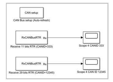
Please open "your CAN Controller library folder"/examples/example1\_receiveRTR.slx (You must change USB serial Port number in CAN\_setup block according to your physical USB port number)
