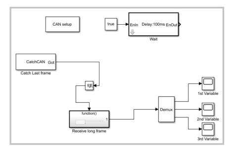
It has "Wait" 100ms block (we make assumption: long frames will be done within 100ms). This "wait" block will lead to actual sampling time=100ms besides simulated sampling time=0.1 sec.
