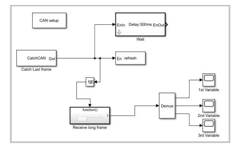
In CAN setup block, we disabled "Auto-refresh" function. And when we caught the last frame of "555" data frames, CatchCAN block will output one pulse. This pulse will give to 3 blocks.
