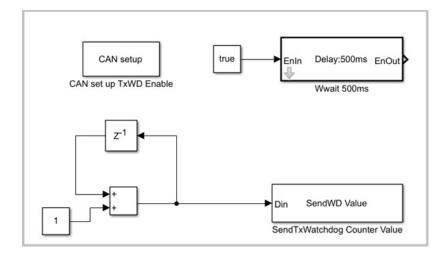
It has "Wait" 500ms block. This "wait" block will lead to actual sampling time=500ms besides simulated sampling time=0.5 sec.
