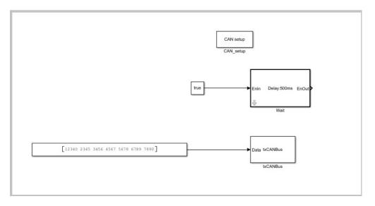
Please open "your CAN Controller library folder"/examples/example2\_transmitLong.slx (You must change USB serial Port number in CAN\_setup block according to your physical USB port number)
