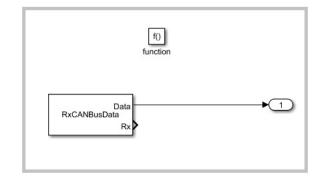
"RxCANBusData" block will get long frames' data output. And at last , we use Demux block to divide vector to 3 variables which are displayed in 3 Scopes.
